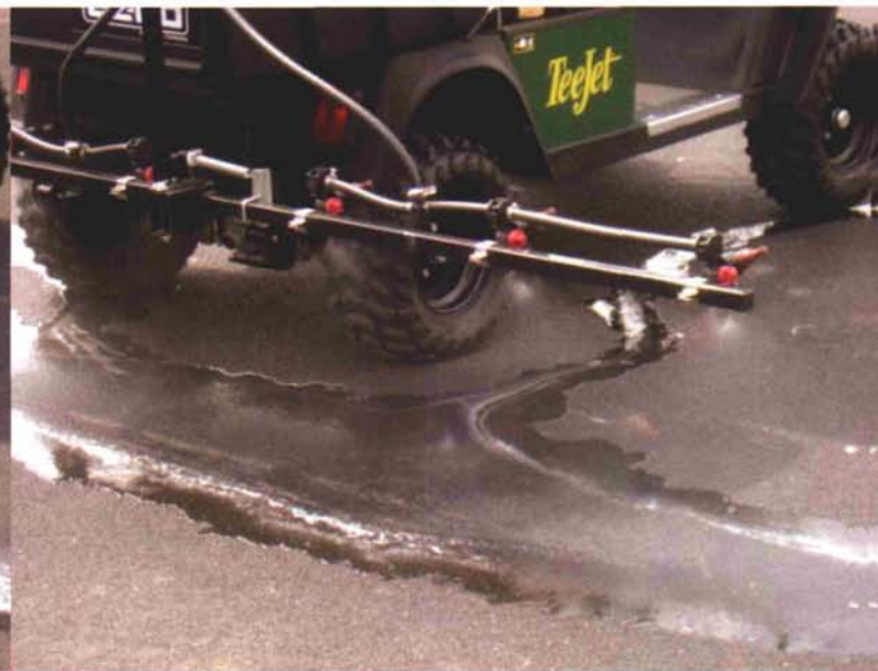
Who says nozzle selection is not important? Notice the coarse droplets on the left compared to the finer spray droplets on the right.
