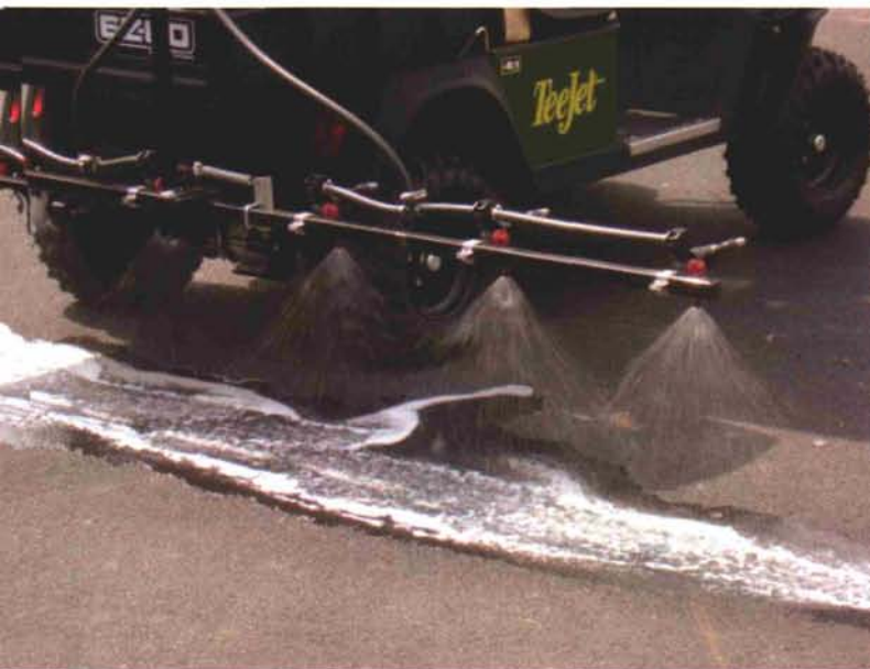
Who says nozzle selection is not important? Notice the coarse droplets on the left compared to the finer spray droplets on the right.
