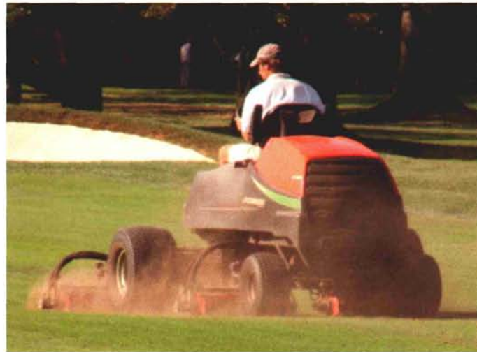
Fairway verticutters are used to clean-up the soil left on the fairways after aeration.
