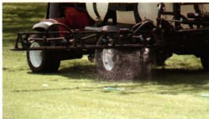
Fig 4. Utilizing GPS technology, sections of the sprayer apply product only to desired target area.
