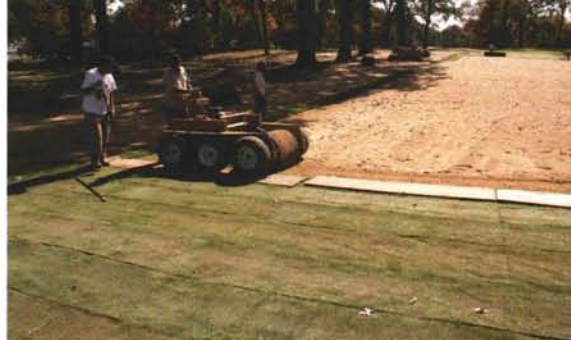
A customized installer for bigroll bentgrass sod.
