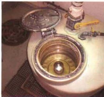
Circulation and agitation of water and product occurs in the 75-gallon mixing tank.
