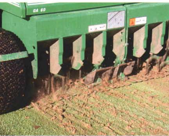
Aerification in process
