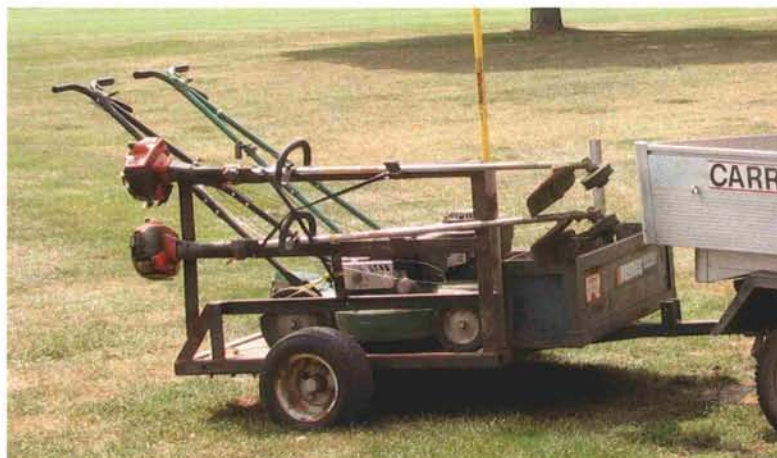
The trim trailer made from an old Dedoes drum aerator.
