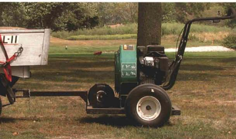
The made-from-scratch blower trailer.
