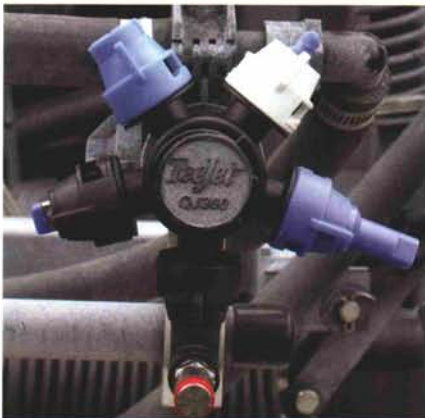
Figure 1. Multiple-nozzle body with five different nozzles.
