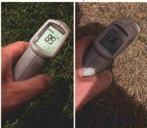
The difference in surface temperature between active, well-irrigated turf and dormant turf is dramatic.
