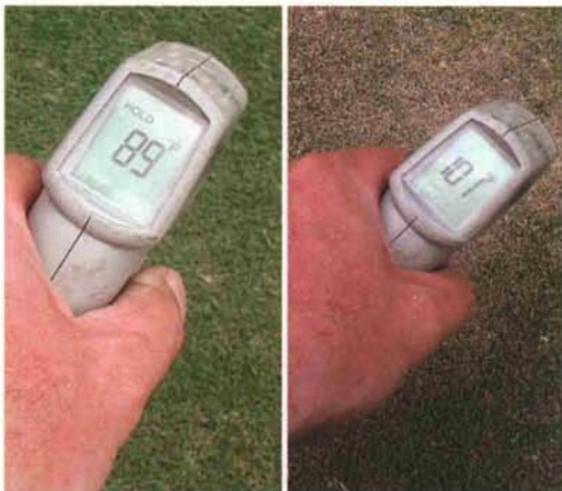
These images of a localized dry spot at North Shore Country Club’s nursery demonstrate the difference in cooling ability (12 degrees) between a functioning plant with proper soil moisture versus a plant under moisture stress from hydrophobic soils.
