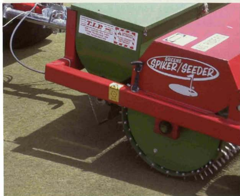
Spike seeding with a machine like this one is perhaps the most popular way of interseeding putting greens in Chicagoland.
