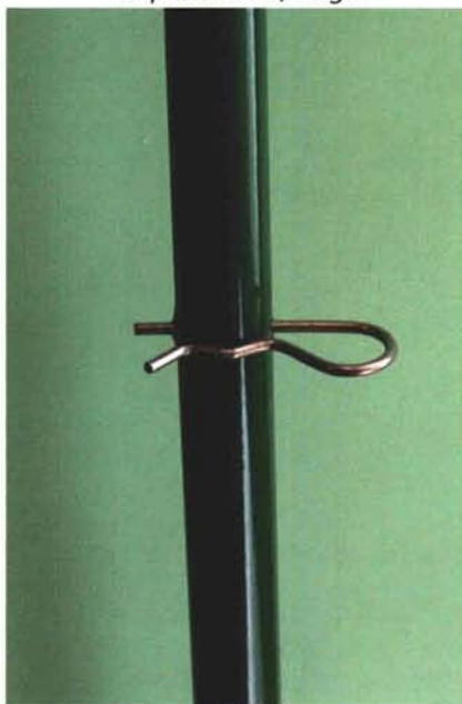
Image 3: Try using a cotter key to hold the placement flag in the correct position.
