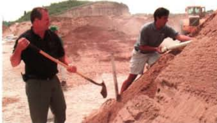
Using the new stockpile-sampling procedure written by Jim Moore, USGA Green Section, Tom Lively and his Course No. 1 assistant collect a sand sample during a visit to a local sand supplier.
