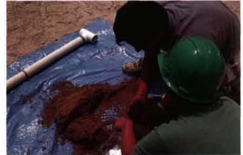
Preparing a representative sample from a large stockpile of sand requires hand-mixing a minimum of eight subsamples. After thorough mixing, a one-gallon sample is sent to a certified physical soil-testing laboratory.
