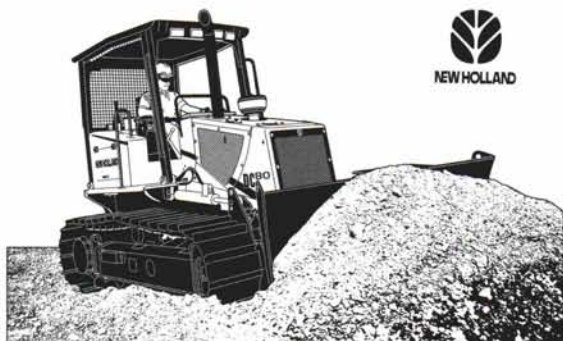
80 hp dozer with hydrostatic transmission and 9'4" blade
