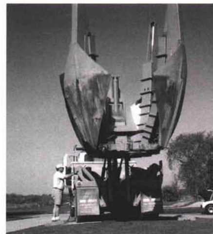
Making room for skyboxes and bleachers around #18 green required moving 12 trees to new sites. Here, a 90” tree spade sets up to take a plug from the lawn for transplanting a ginkgo tree.
