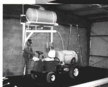
Environmentally correct process to reclaim tainted rinse water. Can be located anywhere
