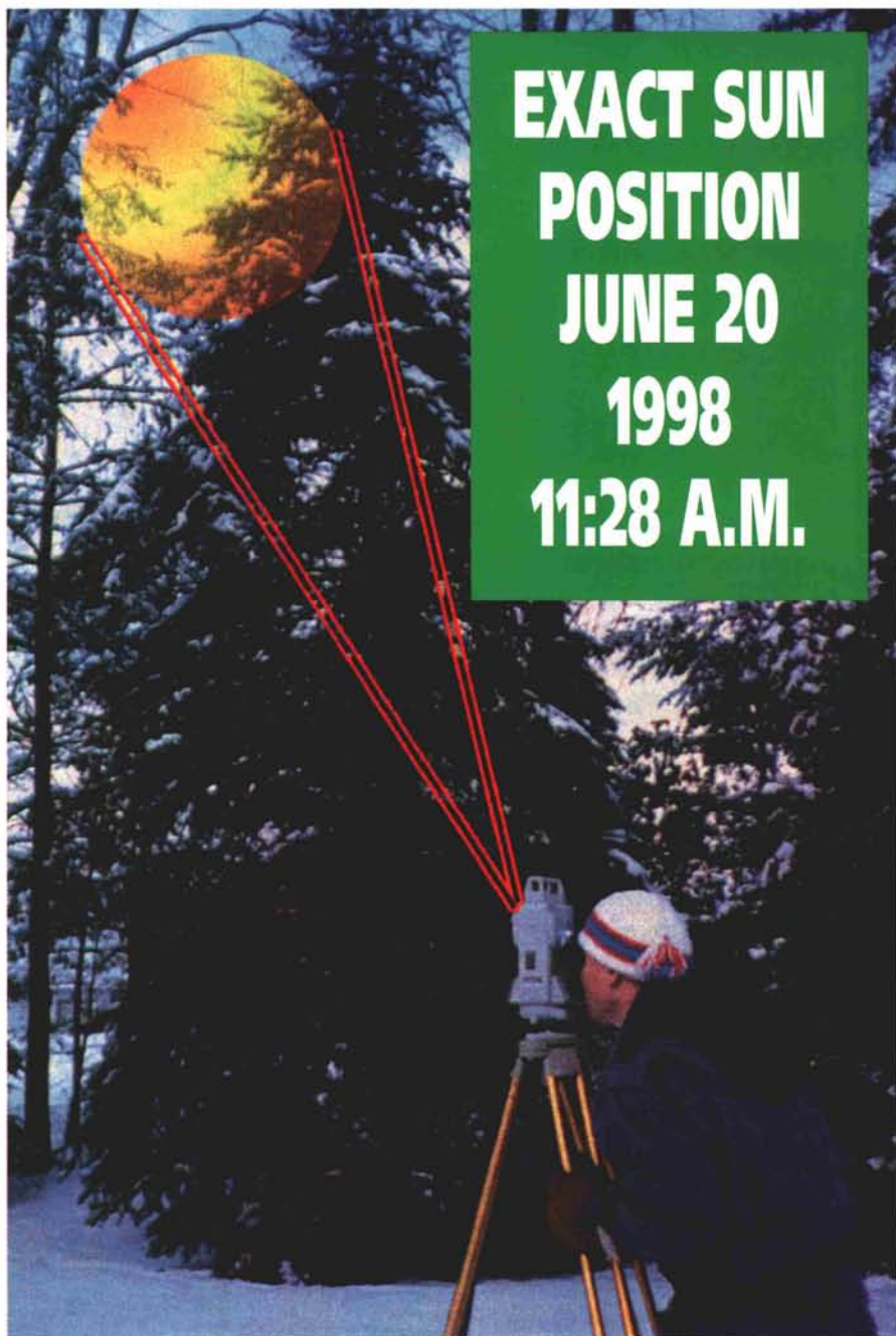
New technology allows the consultant to go onto a golf green in January and determine the position of the center of the sun in June within 1/16 in. at 200 ft. from the sun location instrument.
