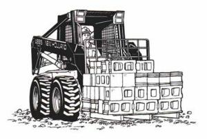
The New Holland Super Boom<sup>™</sup> skid-steer loader will help you be more productive no matter what the application. The long wheelbase makes it more stable so you get better lift capacity than ordinary loaders. And it can go uphill with an empty bucket and come down with a full one.
