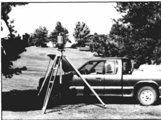
Fig. 2. Laser Transmitter with grade control for use on equipment with automatic laser control.
