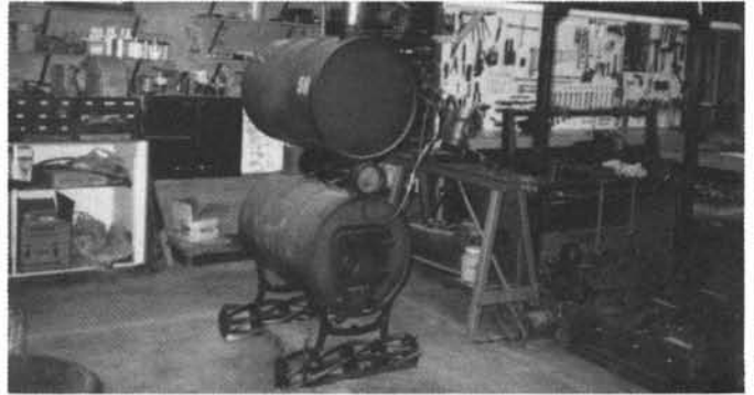
Here is one way to recycle your old reels and save on the energy crunch by burning your brush and logs to heat the shop.
