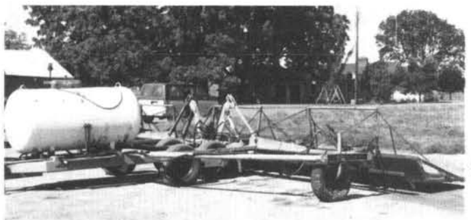
4. A propane burner which burns off the fields at the end of the harvest.
