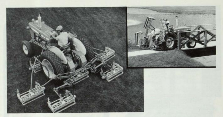
Beginning a new era in turf mowing, the Roseman 7 unit Hydra-Gang Mower utilizes the tractor power take-off system to power the cutting reels and the tractor hydraulic system to provide hydraulic lift for each mower unit. Hills and banks can be mowed easily regardless of soft or wet turf conditions. Individual mower units follow ground contour with unlimited flexibility without scalping. The Hydra-Gang mounts on Ford 2000 and 3000 All Purpose model tractors.
