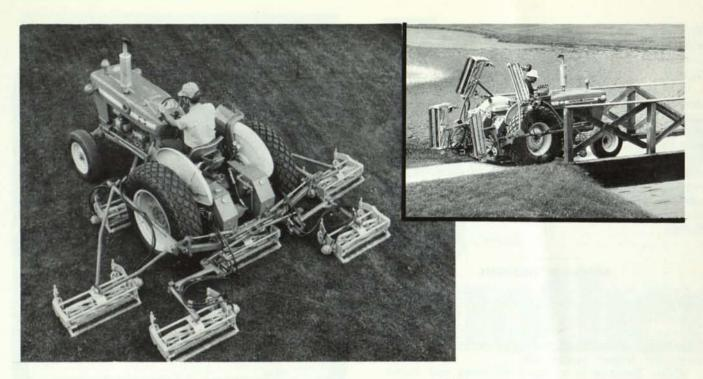
Beginning a new era in turf mowing, the Roseman 7 unit Hydra-Gang Mower utilizes the tractor power takeoff system to power the cutting reels and the tractor hydraulic system to provide hydraulic lift for each mower unit. Hills and banks can be mowed easily regardless of soft or wet turf conditions. Individual mower units follow ground contour with unlimited flexibility without scalping. The Hydra-Gang mounts on Ford 2000 and 3000 All Purpose model tractors.
