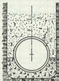
CONCRETE CRADLE BEDDING Load Factor=2.25-3A
