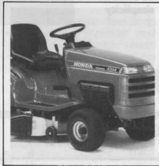
The Honda H4514 lawnmower which is equipped with the Honda 'Slick Shift' hydrostatic stepless shift mechanism.
