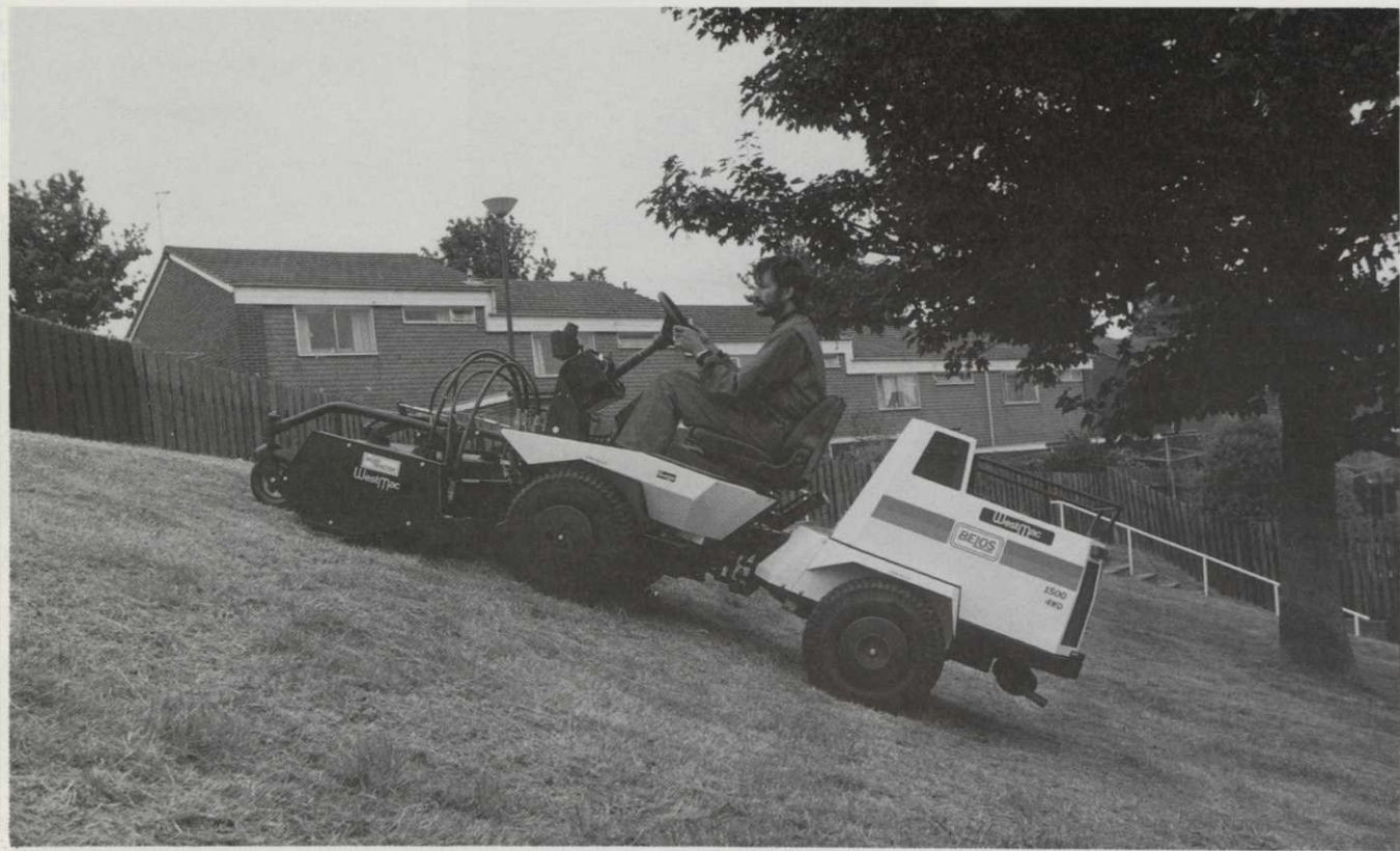
The low centre of gravity of the Belos gives extra stability and safety - especially on slopes.
