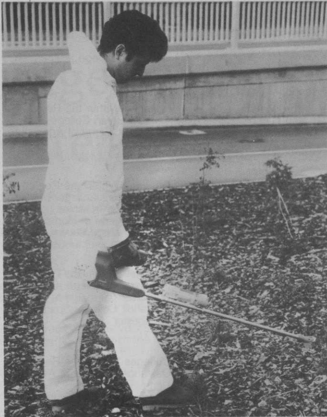
The lightweight Nomix Compact – each chemical cartridge contains enough herbicide to spray for 3 miles.
