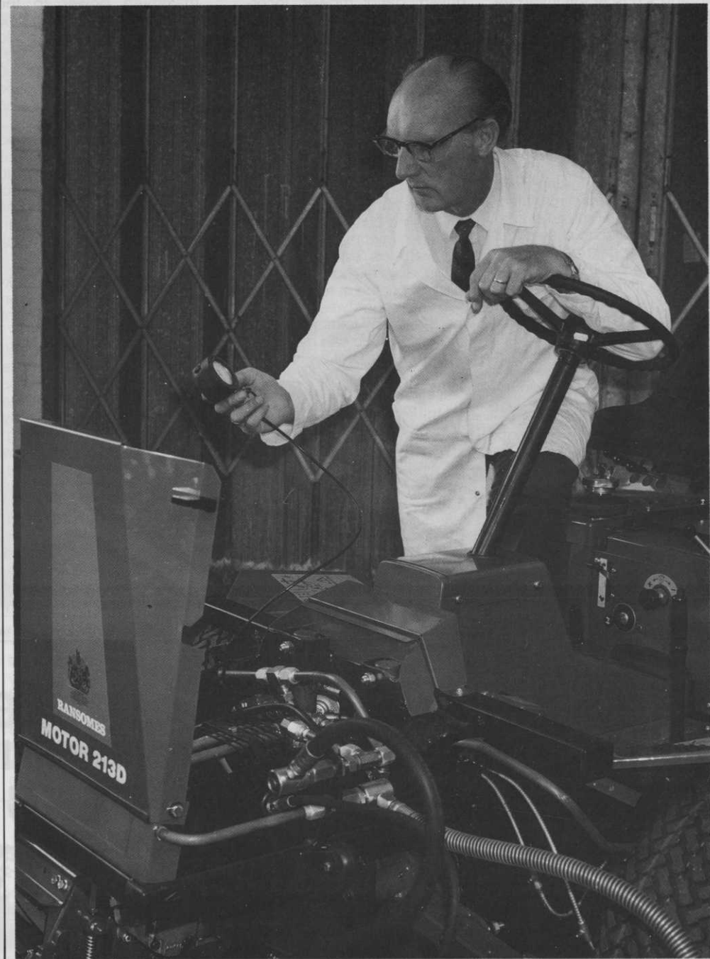
Ransomes Quality Audit Engineer, Mr. Barry Saunders, checking the hydraulic oil pressure while carrying out a quality audit on a triple mower off the production line.
