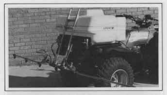
non-drip diaphragm check valves (DCV's) provide a range of application rates with a total swathe width of 4m.
