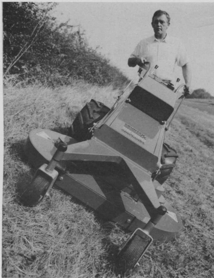
The New Countax CD1200 HDL is a 42in cut, diesel rotary mower with Hydrostatic drive and diff lock.
