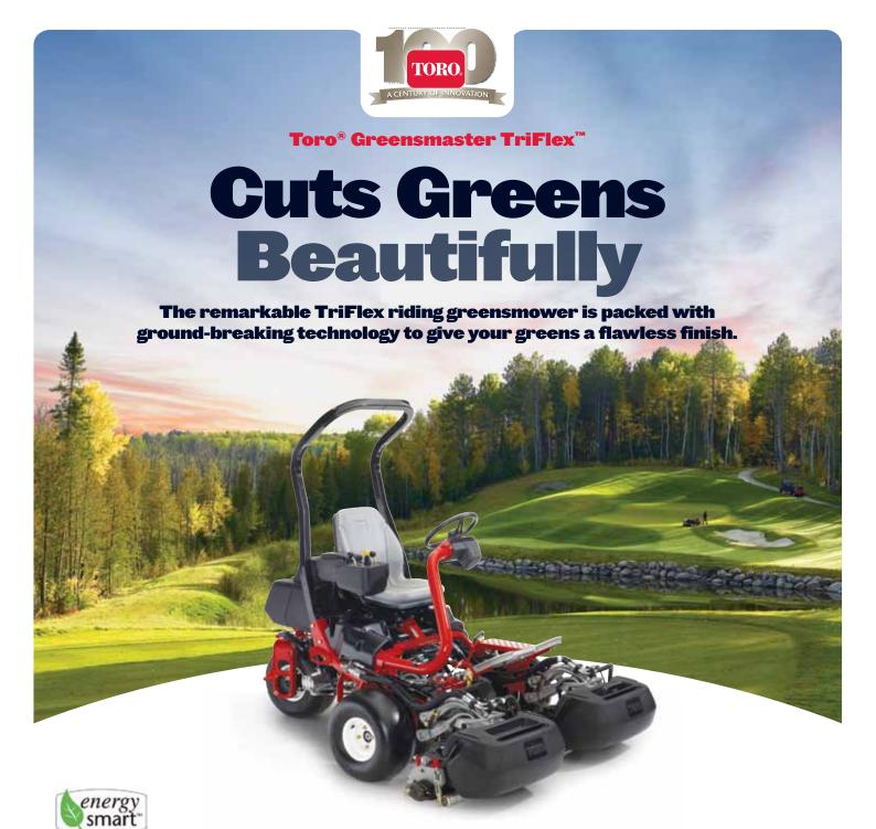
Designed and built from the ground up, the TriFlex range provides unsurpassed consistency and quality of cut. Innovative features, such as Toro's unique Flex double A-arm suspension system, Dual Precision Adjustment (DPA) cutting units and redesigned balloon-style tyres, all combine to produce an outstanding greensmower with the lightest of footprints. What's more, the TriFlex Hybrid 3420 model is the first Toro to feature an all-electric cylinder drive system, for an even greener mower.
