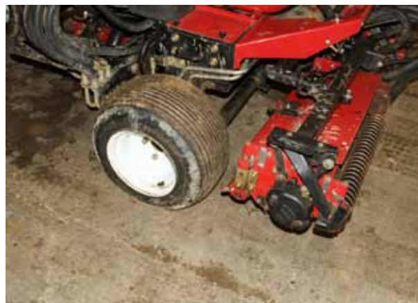
ABOVE: Ribbed tyres have replaced the original turf tyres on one of the Sidewinder mowers. This enables the unit to turn with minimal scuffing when mowing tees
