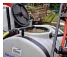
INSET ABOVE: Spray Star sprayers are filled via 41cm diameter hinged lid.
