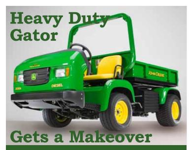
John Deere's 24hp ProGator 2030A diesel utility vehicle has been improved for 2012 with the addition of hydraulic disk brakes on all four wheels for increased performance, and a higher maximum payload capacity of 1594kg.
