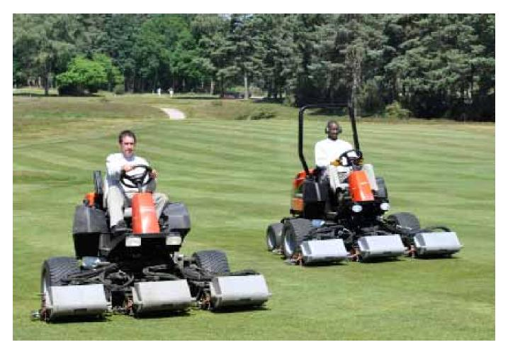
offered, height of cut spanning 2 to 28.5mm dependent upon bottom blade bedknife and roller specified. Those heights of cut are not a typo either, reflecting the use of 'greens' cutting units on a mower that has the width to tackle a wider area.
