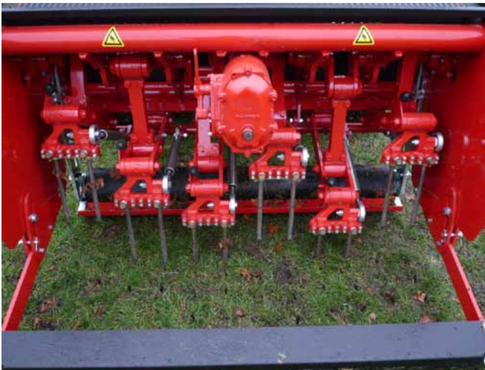
The now ubiquitous Verti-Drain, from Charterhouse Turf Machinery, is designed to relieve deeper compaction. The pictured Verti-Drain 7521 has a 2.10m working width and can operate down to a depth of 400mm. A choice of hollow and solid tines are available.
