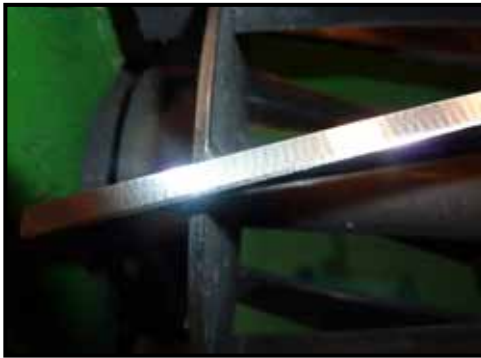
The cutting edge has been relief ground, leaving a slim 1mm thick 'land' on the blade.
