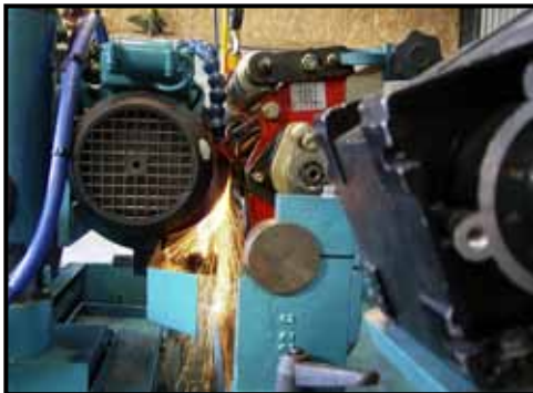
Spin grinding in action, with the cylinder in-situ in the cutting unit.
