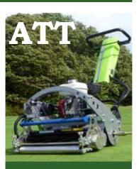
The Grass Group has unveiled the latest development from Advanced Turf Technology offering a progression for the INFiNiPower pedestrian drive unit which will now be available with an all new hybrid petrol/electric power unit. It incorporates a 1.5kw generator, coupled to a Honda GX-120 engine, to deliver a continuous 48V supply to both the traction drive and cutting cylinders' DC Brushless motors.
