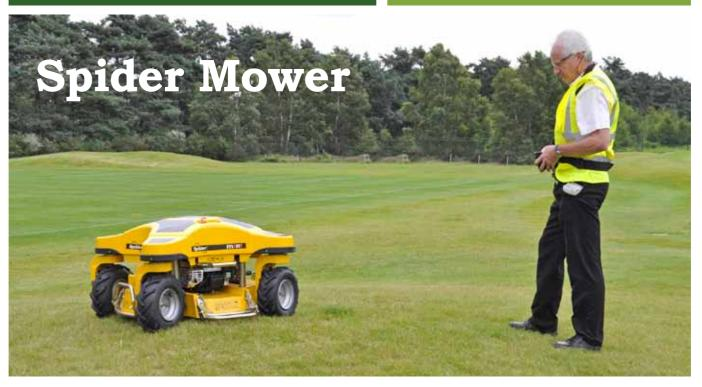
The Ransomes Spider Mini, the latest addition to the range of radio controlled slope mowers, also includes the proven Spider 1 and Spider 2.
