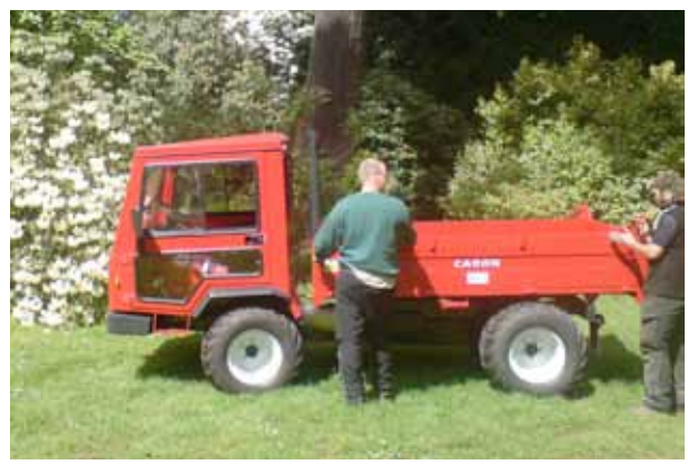
BSG Supplies offer the Caron range of utility vehicles in both single and dual seat variants. If you want a vehicle with a three-way tipping body, adaptable load platform and capacities of 3 tonnes plus, a Caron is worth a look.
