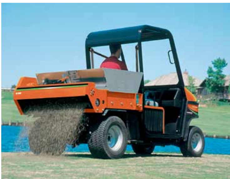
Top dressing is one of those tasks where the spreading equipment can benefit from a low load height. This allows the unit to be filled by hand from a trailer if necessary. A utility vehicle, such as a Turf Truckster, provides the right platform for this type of duty.
