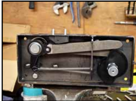
Pictured on the assembly bench at the Vredo factory, the workings of the metering drive can be seen. A key design aim is to ensure low seed rates of small seed, to include Bent grass, can be accurately maintained.
