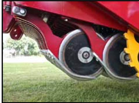
Viewed from the side, the depth of slit can be clearly gauged by the amount of disc protruding through the fingers. The toothed wheel drives the metering unit.
