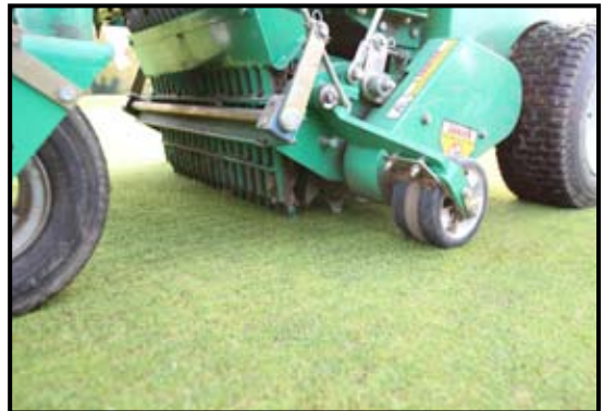
Available in 1mm, 2mm and 3mm widths, the 17 tungsten tipped 210mm blades are spaced at 30mm to give a working width of 510mm. The organic matter removed by the blades needs to be cleared away - a point to consider when working out how long it will take to complete the operation.
