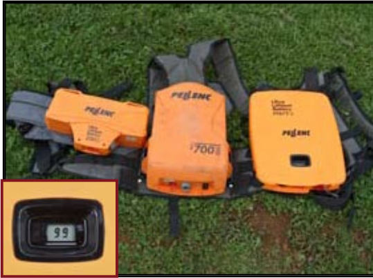
Pellenc equipment is powered by Lithium-ion batteries linked to the tool via a cable. The Poly5 unit on the right represents the latest technology, its 'polymer' design packing more punch into a smaller, lighter package. All feature a capacity indicator. (Inset).
