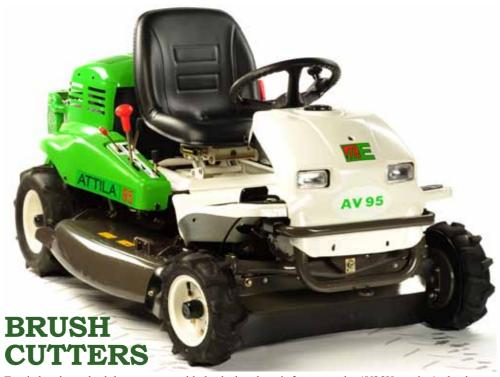
Etesia has launched three new ride-on brushcutters All three models share the distinctive body styling of the Attila AV98 and are powered by Briggs & Stratton Vanguard engines.
