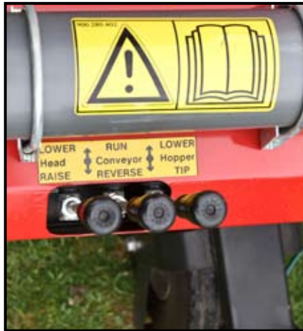
Three hydraulic levers look after the collecting head raise lower, conveyor drive and hopper tip. There is no need to set the collecting head height as it runs on a stainless bottom blade that is designed to 'slide' under the cores. Note sealed tube to house operator handbook.
