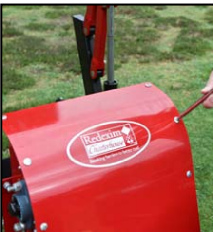
The elevator top cover is secured by six Dzus fasteners and hinges forward to allow easy access to the conveyor for cleaning. The conveyor has external adjusters for tension with greaseable bearings. Keeping the unit clean and lubed is about all the maintenance required.
