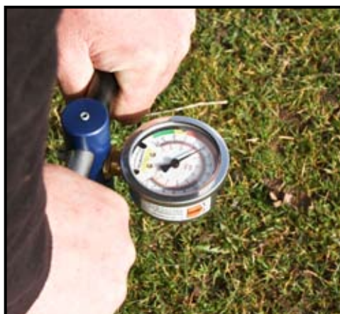
Simple 'before' and 'after' readings from the dial of a Campey Compaction Meter suggest the tool has certainly made it easier to push the probe into the ground.
