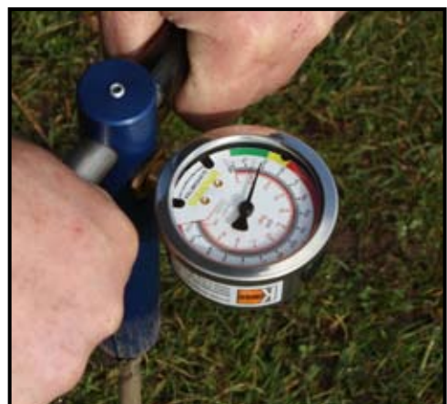
Simple 'before' and 'after' readings from the dial of a Campey Compaction Meter suggest the tool has certainly made it easier to push the probe into the ground.
