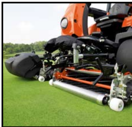
The cutting units come with a choice of options to include groomers...
