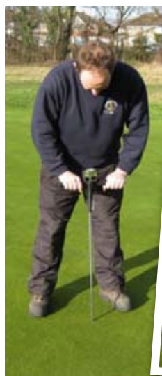
A prism gauge – used to tell the 'true' cutting height.
