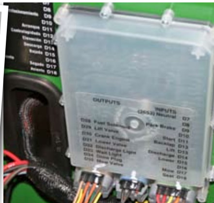
Both 2500 models have Command Arm diagnostic and more advanced 'under hood' diagnostic system. Light pulses will flash in a set sequence to identify key faults, such as a faulty engine glow plug.
