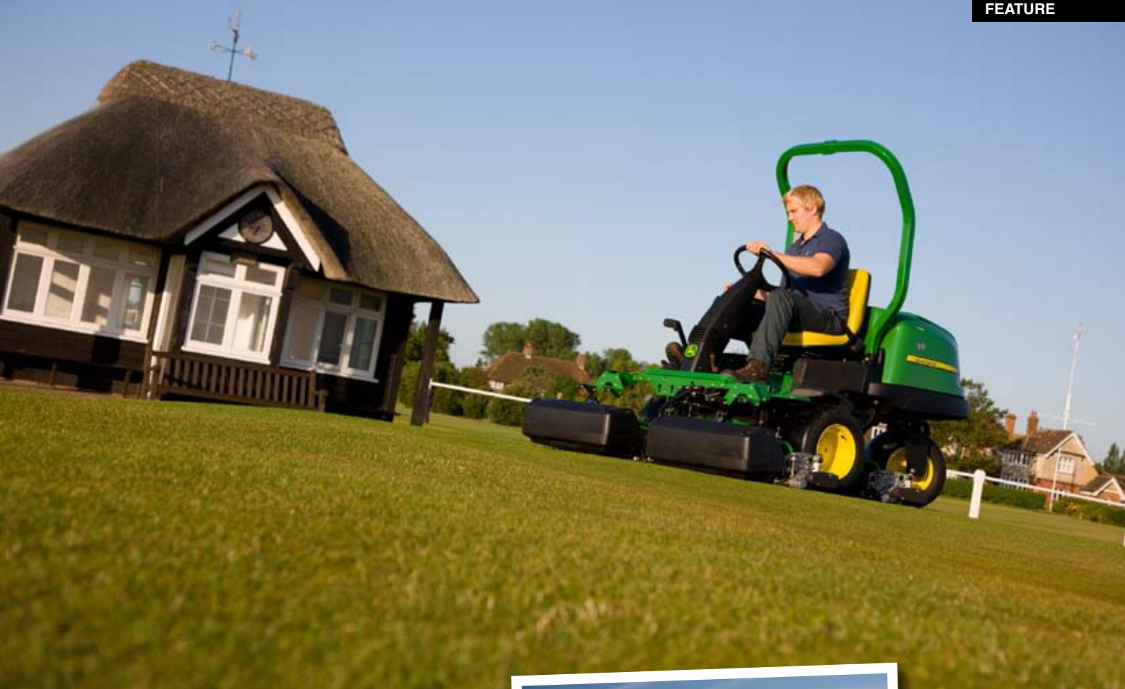
ABOVE AND LEFT: John Deere 2500 greens mowers come in two variants, the 'conventional' all-hydraulic 2500B and 'hybrid' 2500E. This uses a 48 volt alternator to drive brushless electric motors to power the units. The wheels use the same hydraulic system as 2500B.
