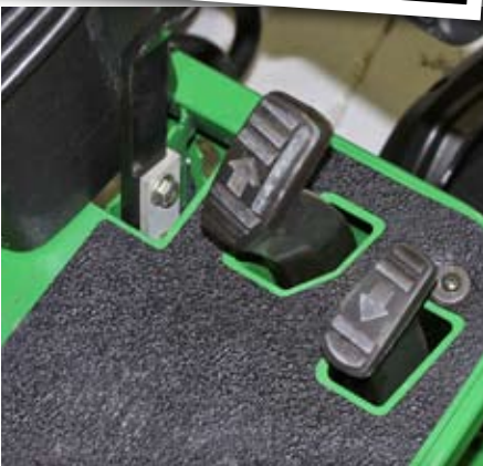
Separate travel pedals feature on both the 2500B and 2500E. As with any item of kit it can take a while to get used to different control types, particularly is you are used to a 'heel and toe' pedal design.
