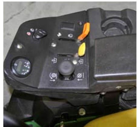
A common control theme is part of Deere's design, the command arm retaining a yellow colour for throttle controls and orange for engaging drive. General ergonomics of Deere mowers is well liked by operators.
