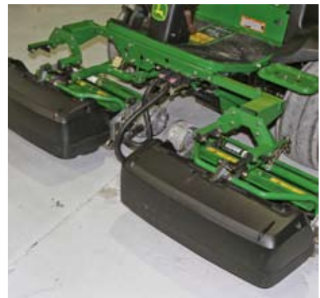
... of 2010 model year 2500 mowers having been refined to ensure even less weight is passed back to the units when the catcher is full.
