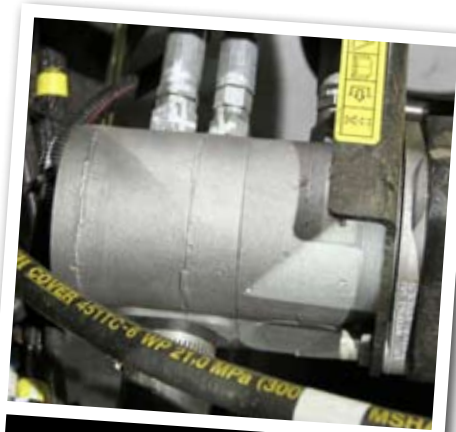
... the 2500B having three independent pumps to power the cutting units, the raise lower function and steering respectively. (continued from previous page)
