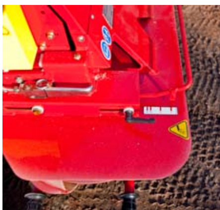
The rear disc carrier adjusts to allow the drop position to be adjusted according to the dressing being applied and the desired spread width. In position 1, this 'Sliding Drop Zone' provides the widest spread width of 9.1m, setting 4 the narrowest at 3.0m.
