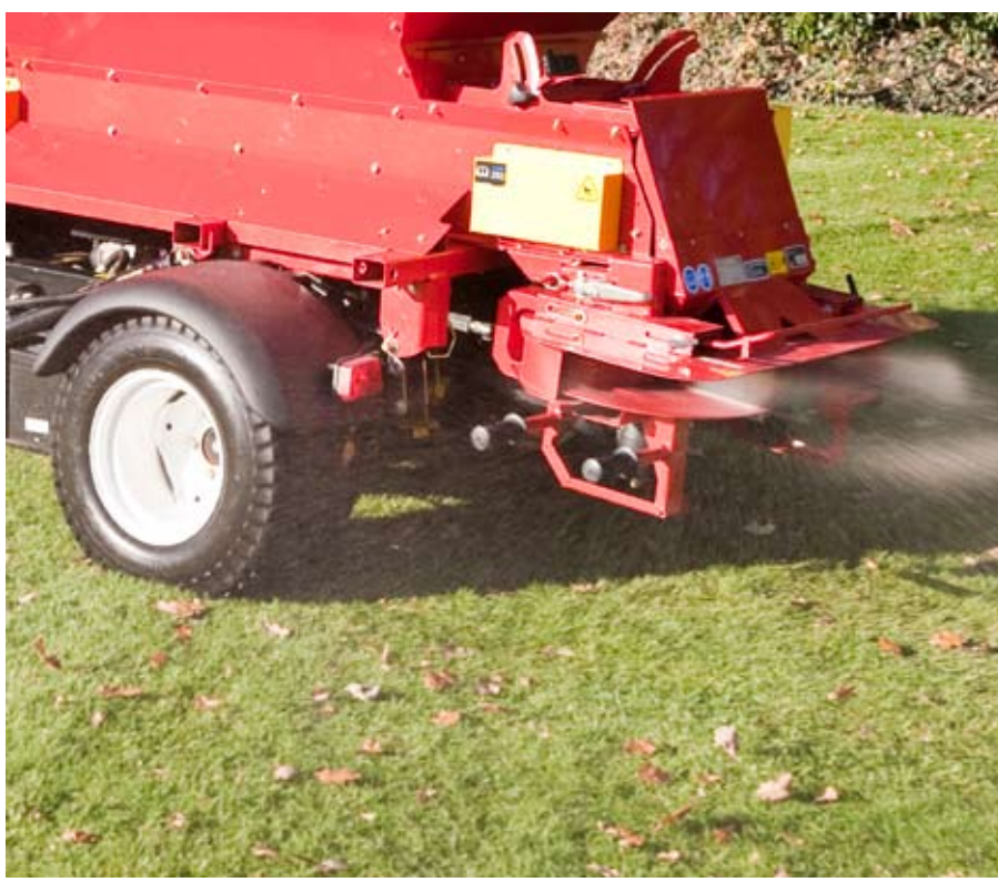
With the optional Wireless Controller, it is possible to fine tune the application rate as the unit is working. This can be useful when the top dressing material moisture levels have changed from when the machine was first set up.
