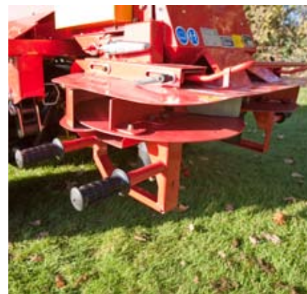
Twin carry handles make it easier to remove the spreading discs either for service or the fitting of a cross conveyor.
