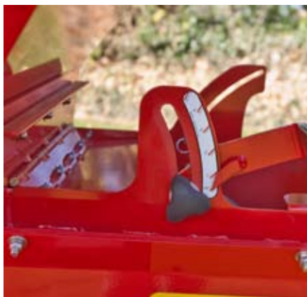
The rate of discharge from the hopper to the conveyor is controlled via an adjustable flap. Base application rate settings are provided by Toro, ease of set-up remaining a ProPass plus.
