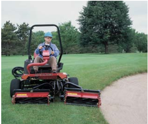
Where the Sidewinder option is specified, all three cutting units can be offset to work 610mm to the left or right. This allows mowing close to vulnerable bunker edges or to be used to alter wheelings around surrounds.
