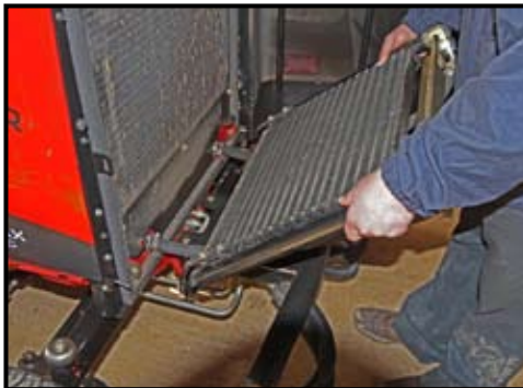
The rear mounted engine radiator and hydraulic cooling package is easy to access for routine cleaning. Positioning the coolers at the rear of the mower helps reduce noise reaching the operator and allows Toro to offer a cab as an option.
