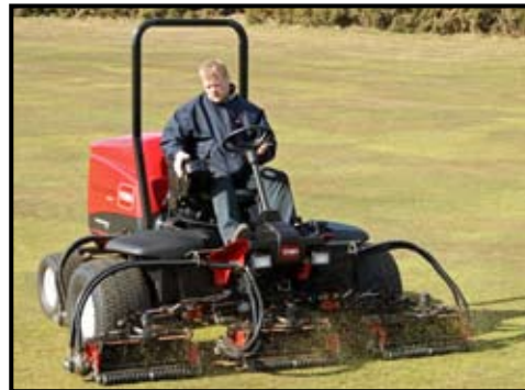
Ribbed front rollers are made of Teflon coated alloy. A choice of groomer or 'groomer broomer' can be specified along with a choice of rear roller scraper or brush. Toro fit their Reelmaster 5410 with 5 inch reels. These are well suited to links and undulating ground.
