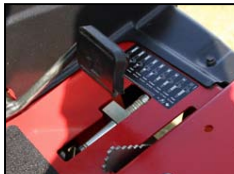
A simple stop if flipped up to limit the maximum mowing speed by limiting the travel pedal. Adjusted by adding or removing washers, the system allows the mower's speed to be easily set in the workshop, the operator flipping the stop down for full travel speed.
