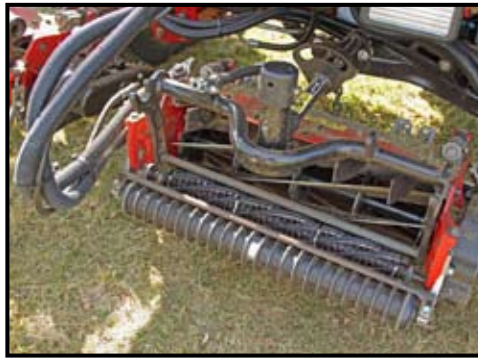
Toro first introduced its DPA - Dual Precision Adjustment - cutting units on its greens mowers, the cast alloy units progressively being introduced to other models including the Reelmaster 5010 series of fairway mowers in 2006.
